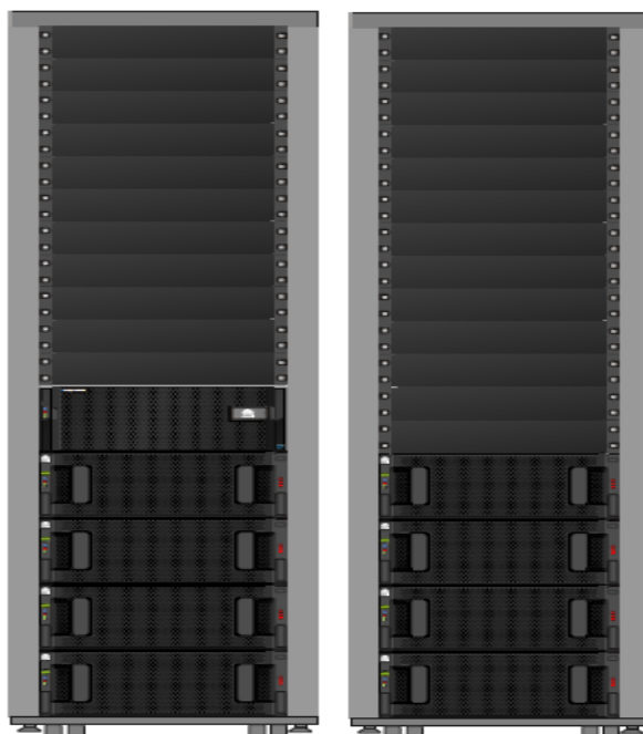
Figure 6-7 Recommended configurations of high-density disk enclosures
